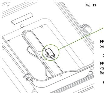
3/16" gap Gas Collector Box - If no spark, pinch together or open Gas Collector Box to adjust 3/16" gap between electrode tip and V-notch.
